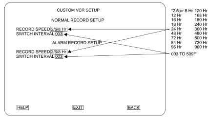
2/6/8 HR FOR NTSC/EIA MODEL MULTIPLEXERS, 3 HR FOR PAL/CCIR MODELS. REMAINING RECORD SPEEDS DEPEND UPON VCR MODEL. VCR TYPE IN RECORD SETUP MENU MUST BE SET TO CUSTOM IN ORDER TO MAKE SELECTIONS.
